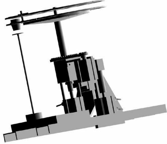
**Dual carousel configuration (for Coal), Fully automatic Placement & Removal of crucible-covers inside furnace**
